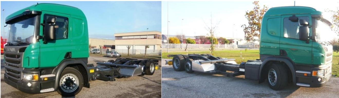
The conversion to a 3 axle chassis as shown above is achieved by commencing with a SCANIA LB 4X2. The chassis frame is lowered in the central area and a fixed (non steer) central axle with on 17,5" wheels is fitted. The axle has pneumatic suspension and is fitted with an automatic lift system with switch control in the cab. The payload on the rear axles with a Tandem load of 16T.
