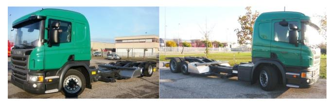
The conversion to a 3 axle chassis as shown above is achieved by commencing with a SCANIA LB 4X2. The chassis frame is lowered in the central area and a fixed (non steer) central axle with on 17,5" wheels is fitted. The axle has pneumatic suspension and is fitted with an automatic lift system with switch control in the cab. The payload on the rear axles with a Tandem load of 16T.
